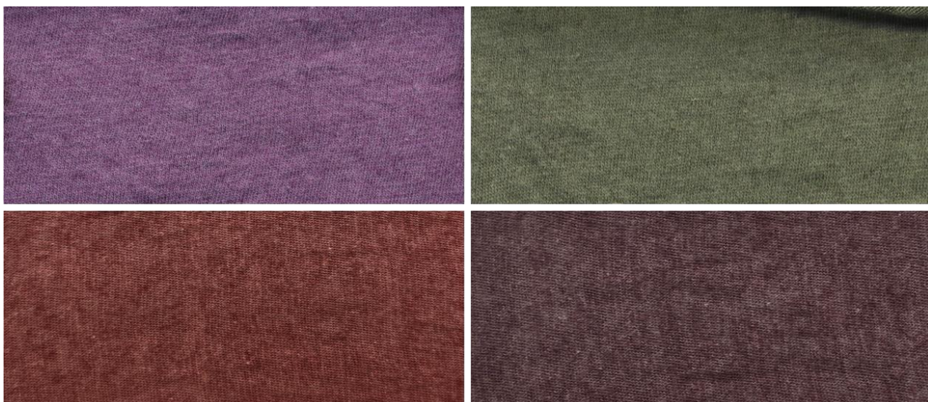
Figure 9. 6% Thiotan R on the 70/30 cotton-ewwools™ fabrics at 1% dye trichromat.
