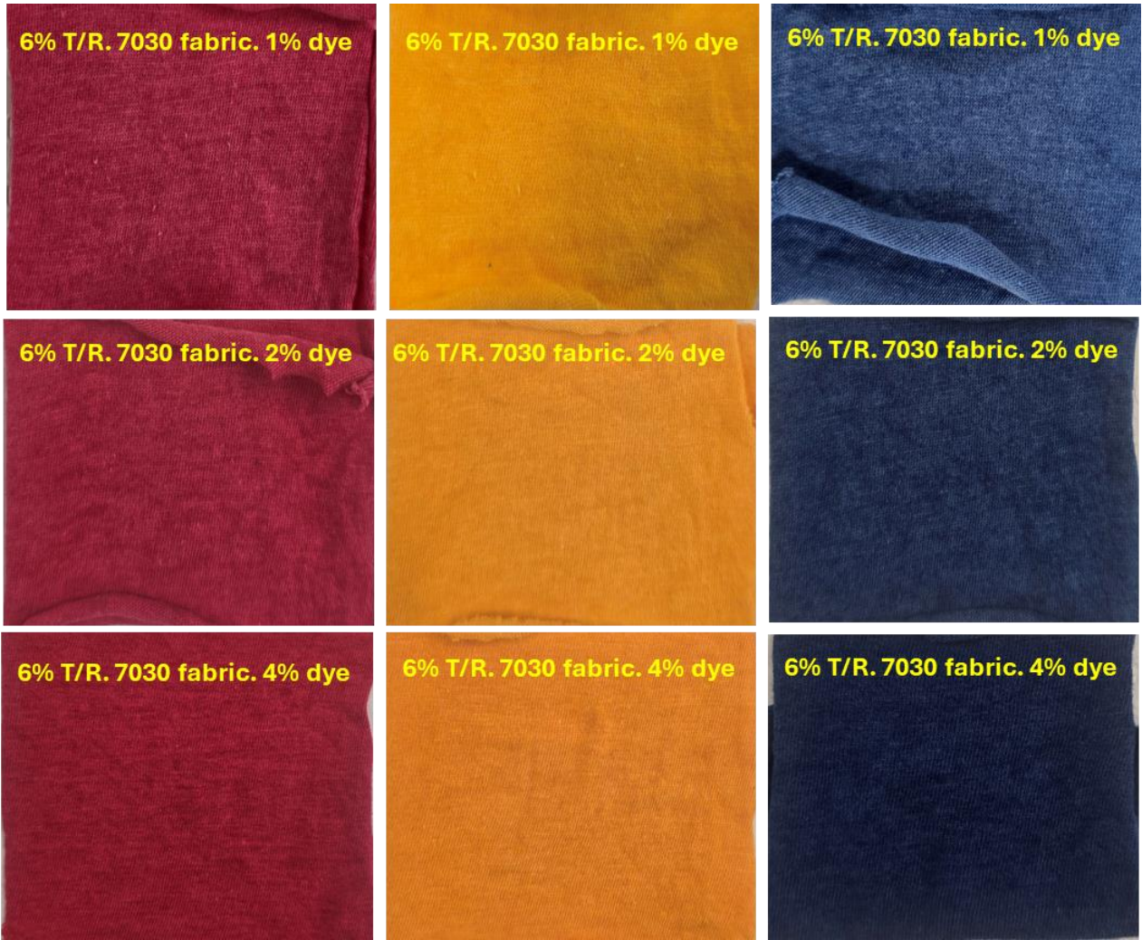
Figure 7. 6% Thiotan R on the 70/30 cotton-ewools™ fabrics at 1%, 2%, and 4% dye.
